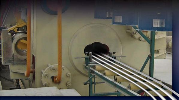
**Anode Rods** are available in diameters ranging from 0.500" to 2.562". Each rod has a steel core running lengthwise through its center. These anodes can be easily configured for various Cathodic Protection applications.
